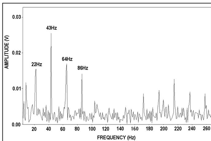
Figure 3: Frequency spectrum of the damaged bearing at 500rpm.
