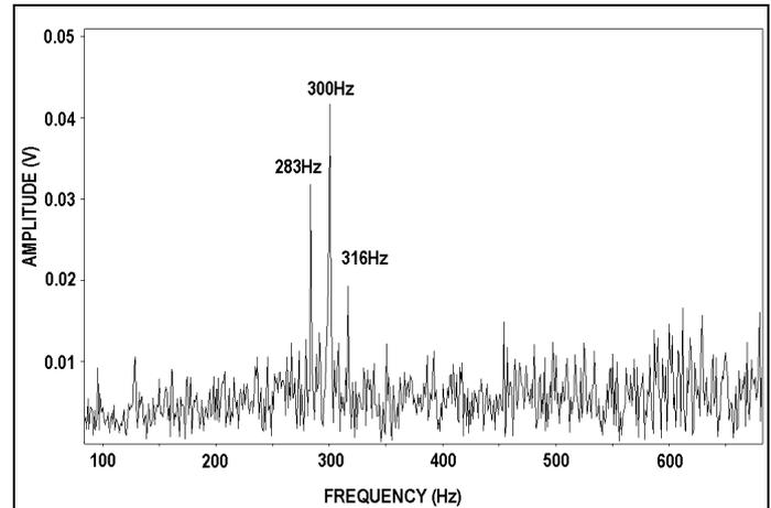
Figure 4: Frequency spectrum of the damaged gear at 500rpm.
