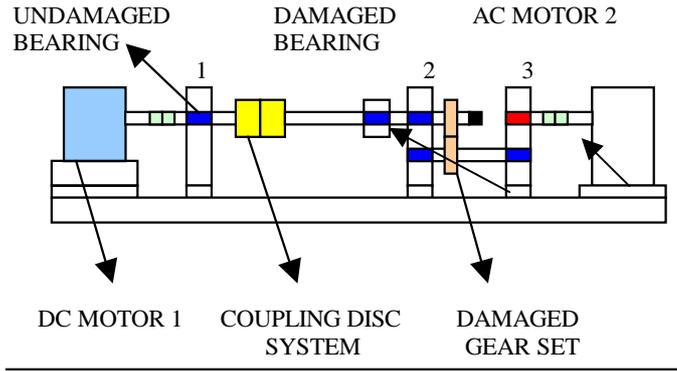
Figure 1a: Schematic of the test rig.
