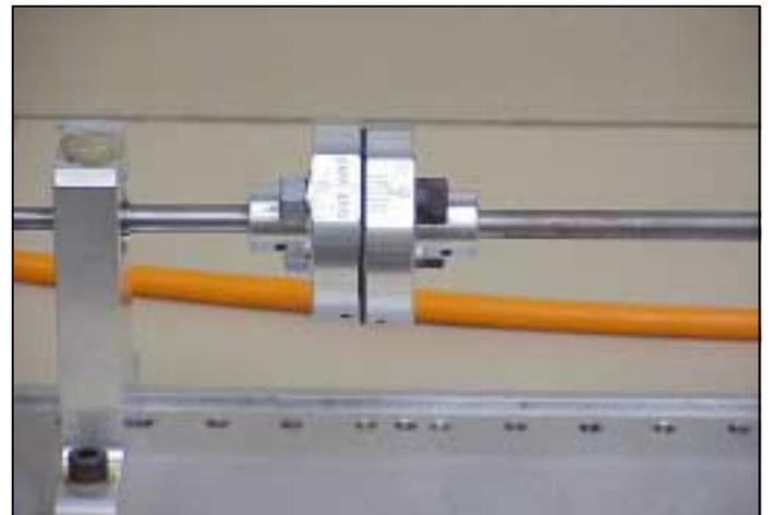
Figure 2: Coupling disc system.
